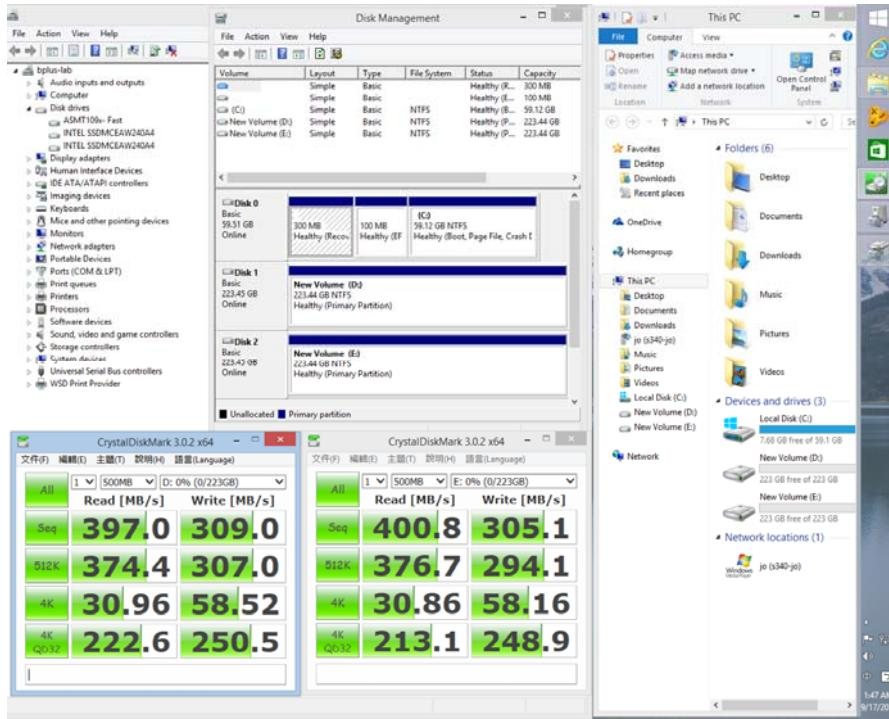
RAID 0: One Disk, consists of striping, Fast, sum of the capacities of the disks
